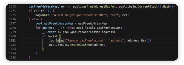
Analyze the function logic of removeGasFree(address), if calling removeGasFree(addr) function, the input-parameter addr will be deleted from both gasFreeAccounts and accounts. But throughout the whole code, accounts will not perform deletion operations, so it is believed that the removeGasFree() operation will cause the account to be out of sync in the two arrays.
