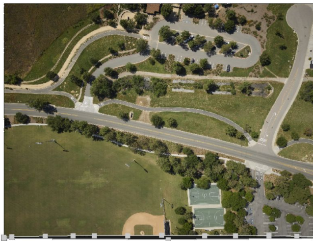
Figure 2.1 A polygon mask outlining the No-Data pixels along the bottom edge of a frame
