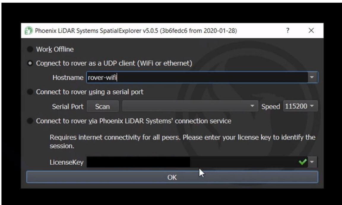
Figure 8: Connect to rover via wifi to test
