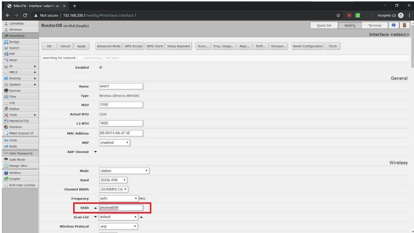
Figure 5: Enter new SSID
